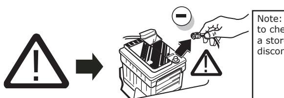
Note: It may be necessary to check if this vehicle has a stored radio code before disconnecting the battery!
